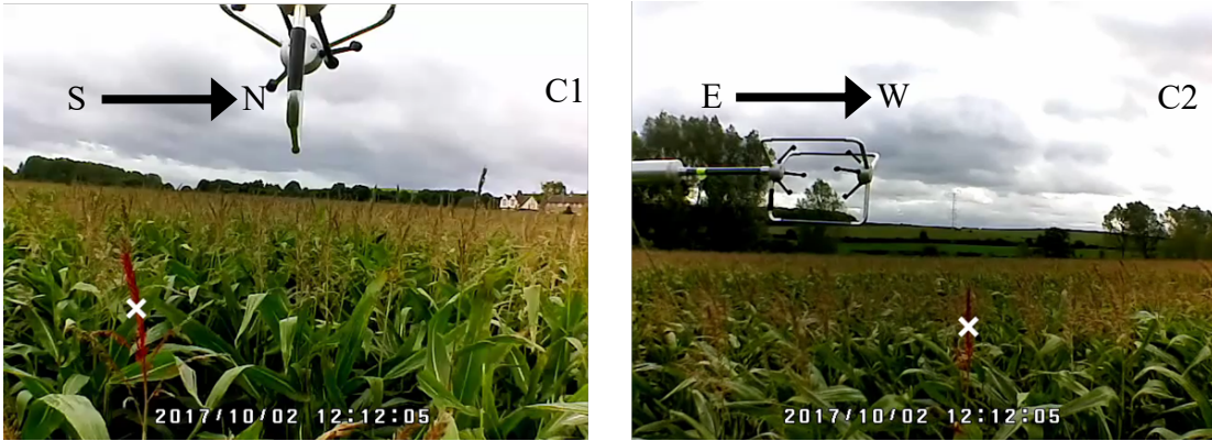
Figure 4 Centroid tracking of maize tassel in a single video frame for each camera, C1 and C2.
